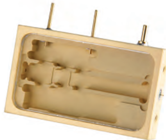
CE11 Hermetic Ka Band Amplifier for satellite application (Tyco M/A-COM)
